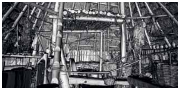
Abb. 4: Die hochauflösende Punktwolke des 3D-Laserscans eines Innenraums. Foto: Arie Kai-Browne The high-resolution point cloud of an interior captured by 3D-laser-scanning.
